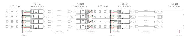
PxLNet Transceivers can also be used to convert two PxLNet data lines to Data + Clock SPI signals. For this option a dual Transceiver setup is required.
