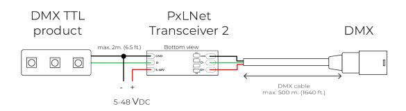
**Note:** These wiring schemes do not necessarily show correct powering your LED products. All wiring schemes in this manual are for reference only, please refer to the technical information or user manual of your LED product, supplied by the manufacturer.
