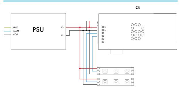
Each SPI Ground wire must be the same length as the Data wires per output, to prevent timing issues. This automatically taken care of when these wires recombined in a single cable. Minor differences in length due to uneven stripping of the wires, should not cause any problems.
