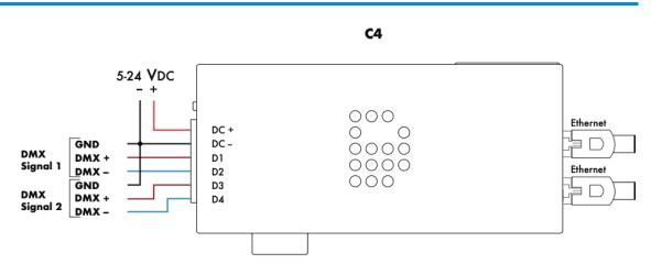
Max. 512 channels per combined DMX port | DMX cable max 500 m. (1640 ft.)
