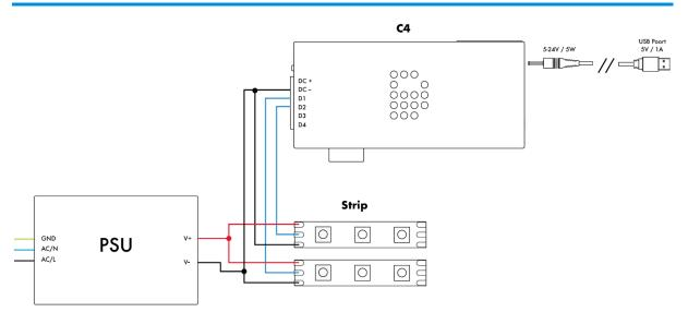
If DC Jack is connected for powering the DiGidot C4, the grounds between PSU and DiGidot C4 need to be connected.
