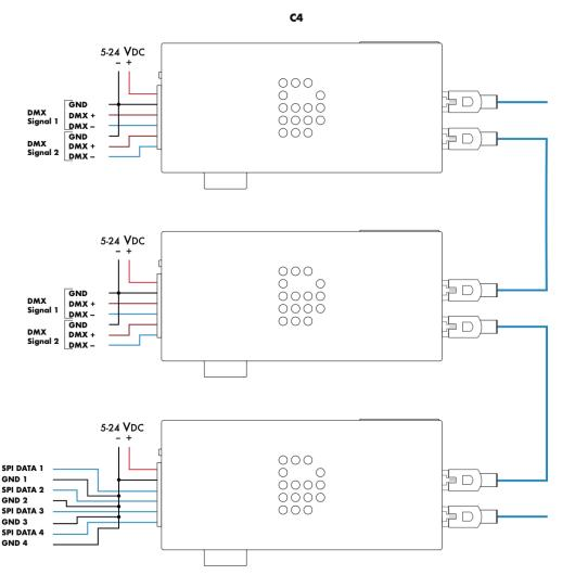
Average recommendation is max. 3 SPI universes per port (check the C4 Performance guide for max. load per IC) | Cable max 2 m. (7 ft.) DMX max. 512 channels per combined DMX port | DMX cable max. 500 m. (1640 ft.)
