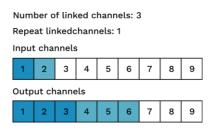
Increase pixel size/ decrease channels: Combine/group multiple output channels into one, in order to save input channels.
