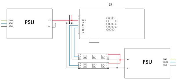
Each SPI Ground wire must be the same length as the Data wires per output, to prevent timing issues. In this case the power supplies grounds do not need to be connected because they share the ground through the LED product.
