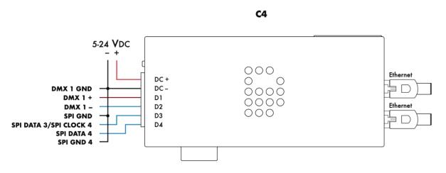
Max. 512 channels per combined DMX port | DMX cable length max. 500 m. (1640 ft.) | SPI cable length max. 2 m. (7 ft.)
