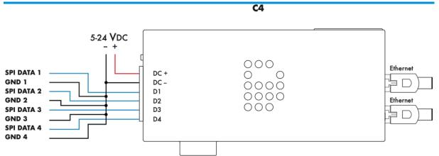
Average recommendation is max. 3 SPI universes per port (check the C4 Performance guide for max. load per IC) | SPI cable length max. 2 m. (7 ft.)
