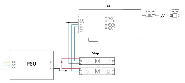
If DC Jack is connected for powering the C4, the grounds between PSU and C4 need to be connected.
