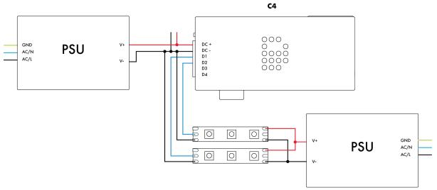
Each SPI Ground wire must be the same length as the Data wires per output, to prevent timing issues. In this case the power supplies grounds do not need to be connected because they share the ground through the LED product.
