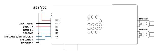
Max. 512 channels per combined DMX port | DMX cable length max. 500 m. (1640 ft.) | SPI cable length max. 2 m. (7 ft.)
