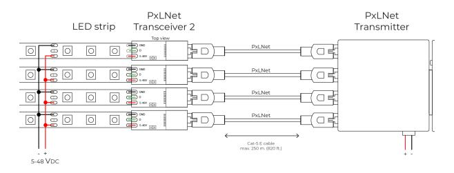
DiGidot C4 with PxLNet Transmitter connected by Cat-5E network cables which are soldered to PxLNet Transceivers which are soldered directly to a pixel controlled LED product.
