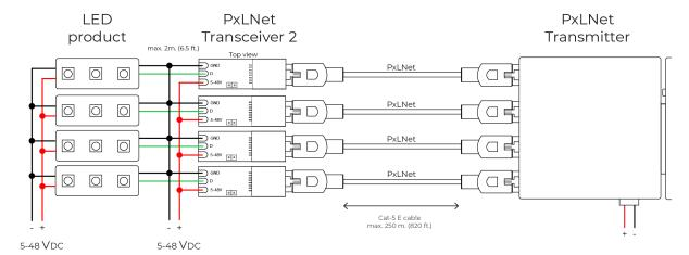
DiGidot C4 with PxLNet Transmitter connected by Cat-5E network cables to PxLNet Transceivers which are soldered directly to a pixel controlled LED strip. At the end of every LED strip another PxLNet Transceiver is placed in transmit mode, to send the remaining signal to the next LED strip. Please note that the operating mode jumper [5] on the top side must be removed to change it to transmit (Tx) mode.
