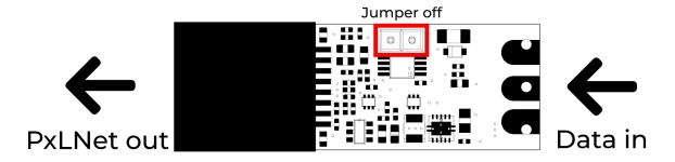
Connect a network cable to the RJ45 bus and connect it to the next PxLNet Transceiver in receiving mode (Rx).
