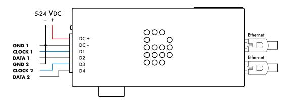
This option shows two SPI Data + Clock signals. Please note that all grounds must be connected.
