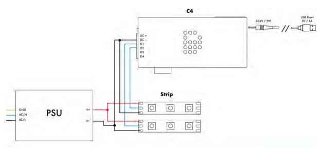
If DC Jack is connected for powering the C4, the grounds between PSU and C4 need to be connected.
