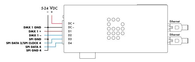
This option shows a combined output of SPI and DMX in or out. Please note that the SPI type (Data only or Data + Clock) determines how you need to connect the SPI signal(s). A Data + Clock signal always requires two outputs of the C4. Cable should be DMX cable with an impedance of 110 Ohm or CAT5 or higher.
