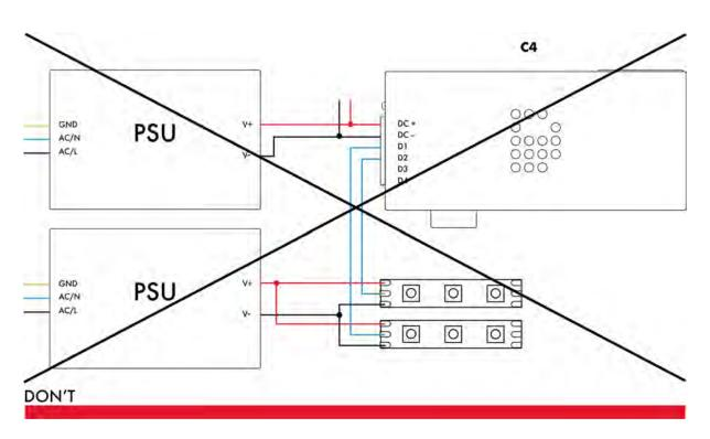
Grounds are not connected and not the same length as the data wires.
