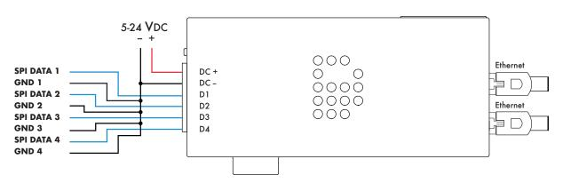
This option shows four SPI Data only outputs. Each SPI Ground wire must be the same length as the Data wires per output, to prevent timing issues.
