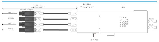
Transmitter connected to DiGidot DMX adapters, by Cat-5E network cables, to get four balanced DMX outputs.
