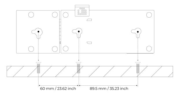
3. Position the mounting holes of both devices over the screws and slide them in place.
