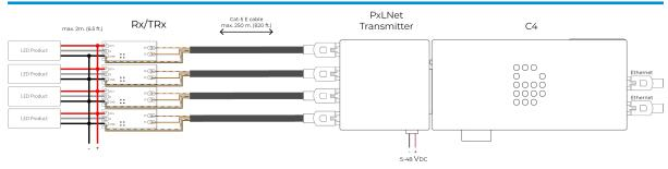
Transmitter connected to Rx48 receivers by Cat-5E network cables that are soldered to the receivers, which in turn have wires soldered to them that go to the LED products.
