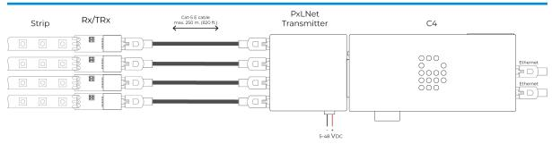
DiGidot C4 with PxLNet Transmitter connected to Rx48 receivers by Cat-5E network cables that are plugged into the receivers RJ45 busing that are soldered directly to pixel controlled LED strips.
