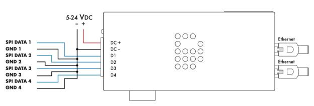
Average recommendation is max. 3 SPI universes per port (check the C4 Performance guide for max. load per IC) | SPI cable length max. 2 m. (7 ft.)
