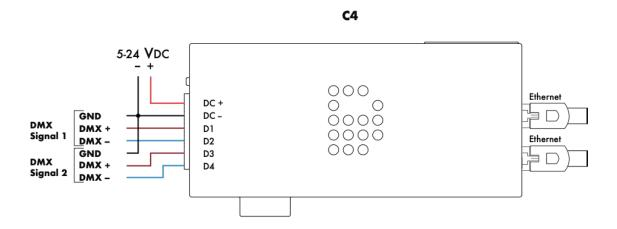
Max. 512 channels per combined DMX port | DMX cable max 500 m. (1640 ft.)
