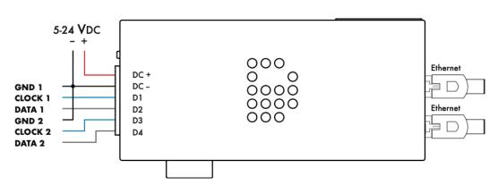
Average recommendation is max. 6 SPI universes per port (check the C4 Performance guide for max. load per IC) | SPI cable length max. 2 m. (7 ft.)
